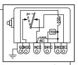
**M4264 Series** Detects loss of magneto/CD ignition output and transfers contacts for customer use. Contacts 10 amps; 48 VAC/VDC.
